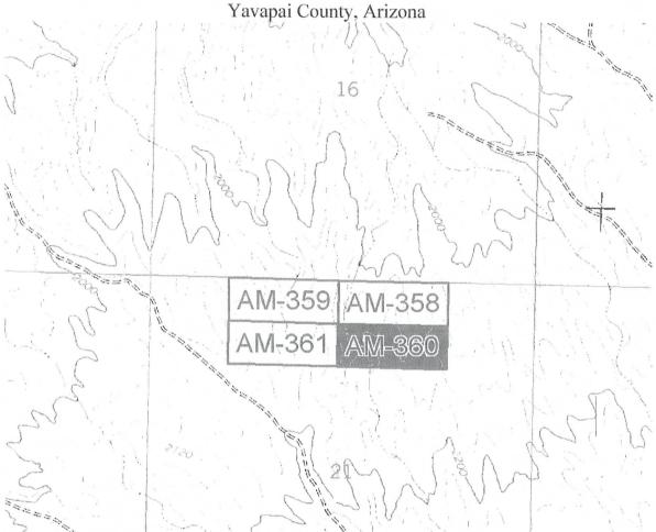
AM-360 Is delineated thusly: From NW corner, 1500 feet at approximately  $90^{\circ}$  to the NE corner, then 600 feet at approximately  $180^{\circ}$  to the SE Corner, then 1500 feet at approximately  $270^{\circ}$  to the SW corner, then 600 feet at approximately  $0^{\circ}$  to the point of beginning.
