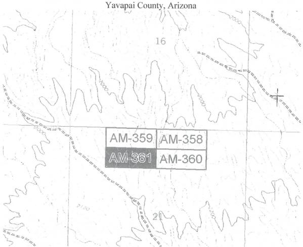
AM-361 Is delineated thusly: From NW corner, 1500 feet at approximately  $90^{\circ}$  to the NE corner, then 600 feet at approximately  $180^{\circ}$  to the SE Corner, then 1500 feet at approximately  $270^{\circ}$  to the SW corner, then 600 feet at approximately  $0^{\circ}$  to the point of beginning.
