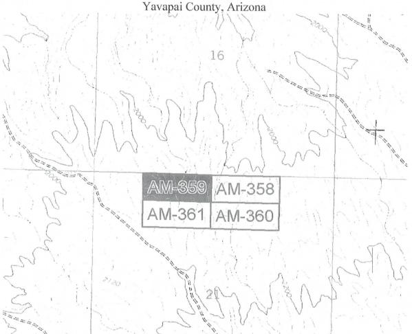
AM-359 Is delineated thusly: From NW corner, 1500 feet at approximately  $90^{0}$  to the NE corner, then 600 feet at approximately  $180^{0}$  to the SE Corner, then 1500 feet at approximately  $270^{0}$  to the SW corner, then 600 feet at approximately  $0^{0}$  to the point of beginning.
